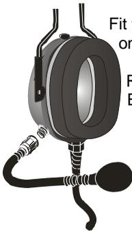
Fit the Microphone Boom assembly to the mounting socket located on the **Right Side** Ear Cup (cable side).
